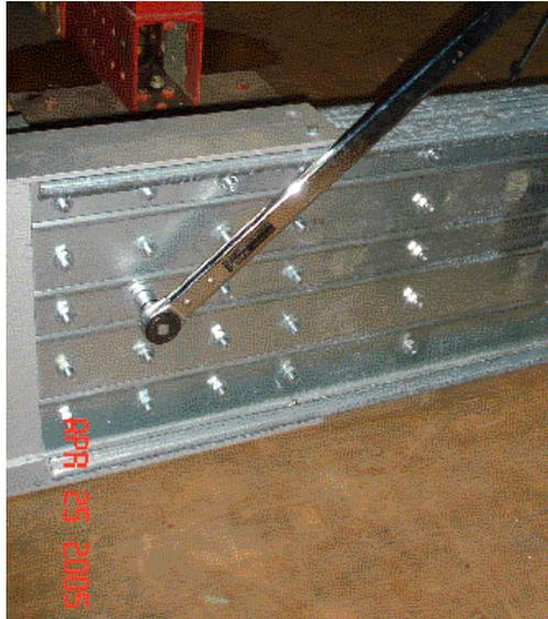
Fig.1 Classic joint connected with HSF bolts
