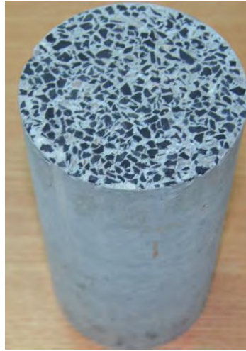
Figure 1. Cylinders made of concrete and rubber
