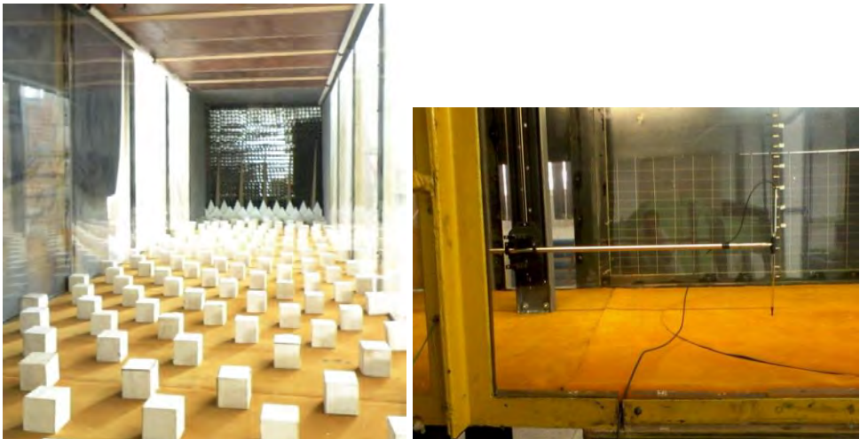
Fig. 3 View inside the BLWT: a) system for generating the turbulence of the flow over an II category of terrain; b) equipment for acquisition of wind velocity
