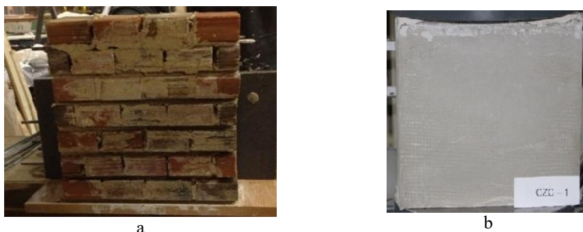
Figure 1. Old masonry samples: a- simple unstrengthened masonry; b- glass fiber reinforced mineral composite samples
