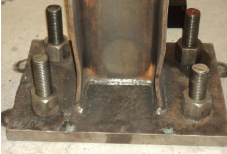
Figure 10. Plastic hinge formation in the column
