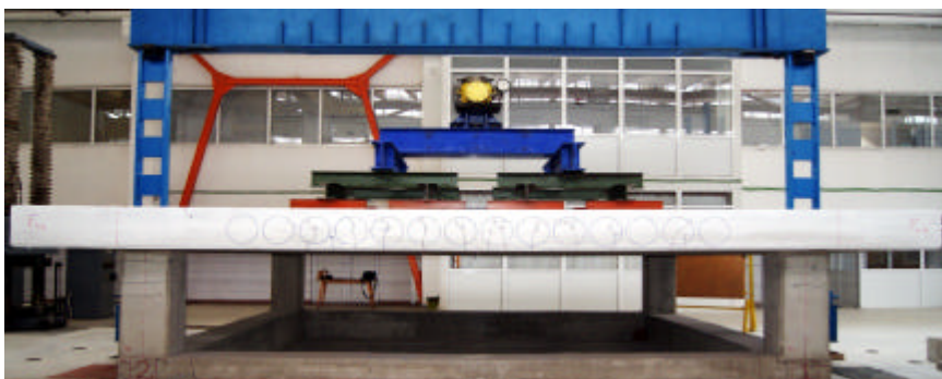
Figure 17. Experimental Crack Patterns, Ax 2-1
