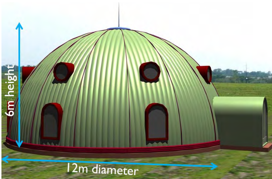
Fig. 3 Perspective view of the structure
