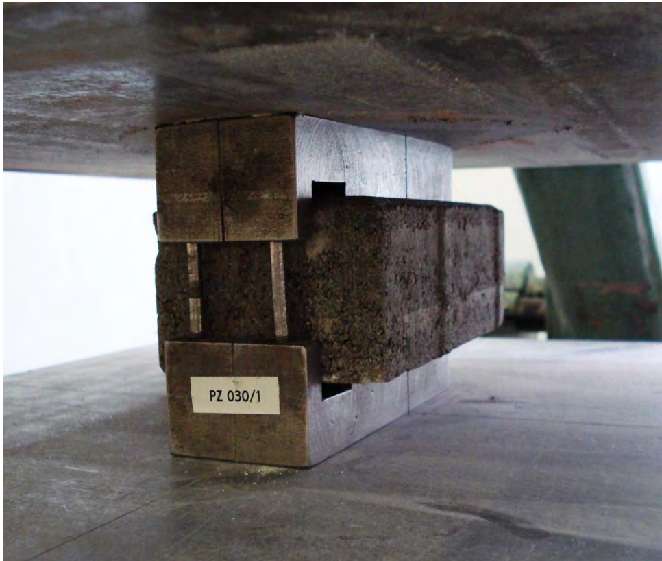
Figure 2. Paving block compressive strength test according to CSN 73 6131-1
