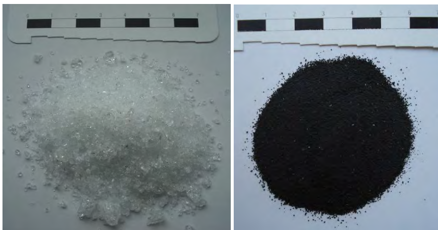
Figure 5, 6. Borosilicate granulated glass (left - Fig. 5.) and fire sand (right - Fig. 6.)
