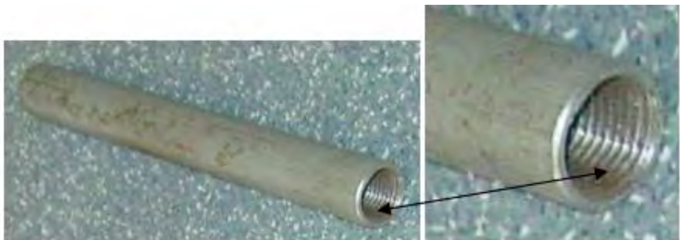
Figure 2. Anchor interior surface mechanical treatment
