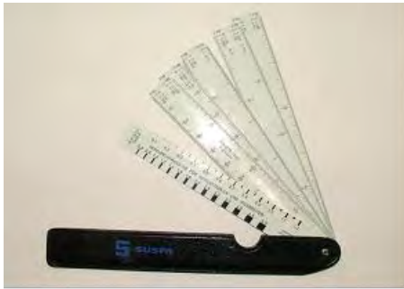
Figure 3. Example of gauge for determining the width of cracking
