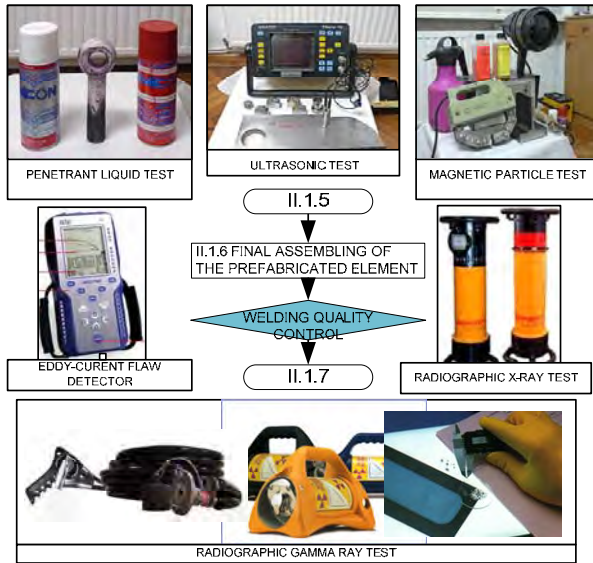
Fig. 21 Specific Equipment for Welding Quality Control
