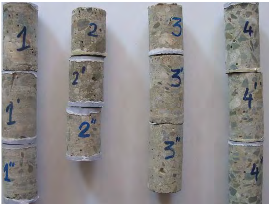
Figure 6. Concrete test rods from the superstructure
