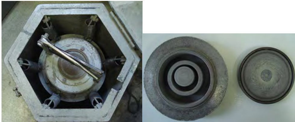
Figure 2. Sight to vibrating mill mouth (left) and grinding chamber with medium (right)
