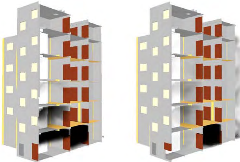
Figure 4. FDS Slice - Image of the two simulations at 140 s fire time. Only smoke visible. Standard simulation (left), and PPV one (at the right side of the figure)
