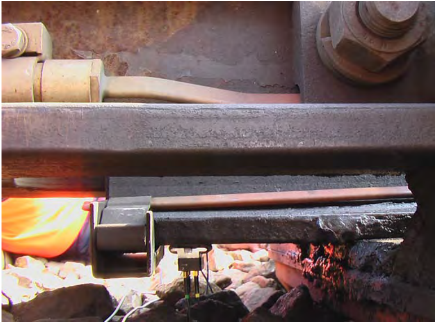
Figure 2. Experimental set up of 3 axis sensor
