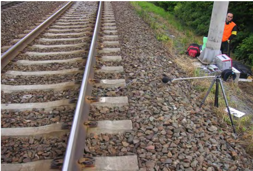
Figure 3 Sensors location, the elastic rail fastening Pandrol FC
