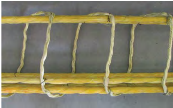
Figure 5. Shear reinforcement shaped into spiral
