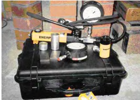
Fig.4. Flat-Jacks Shear Starter Kit
