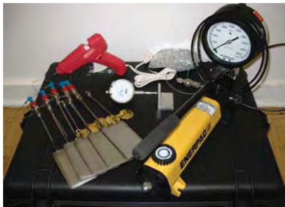
Fig.3. Flat-Jacks Compressive Starter Kit
