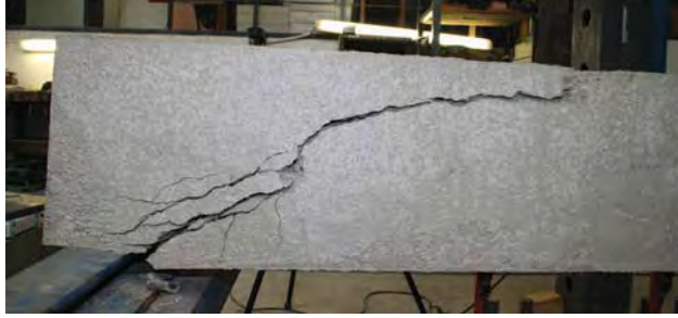
Figure 6. Cracked beam with GFRP shear reinforcement
