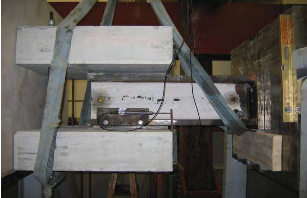
Fig. 2 Complete push-out-specimen ready for testing
