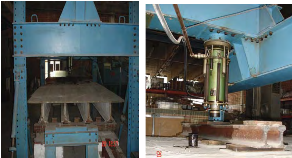
Figure 2. The stand for dynamic testing of bridge models at great scale
