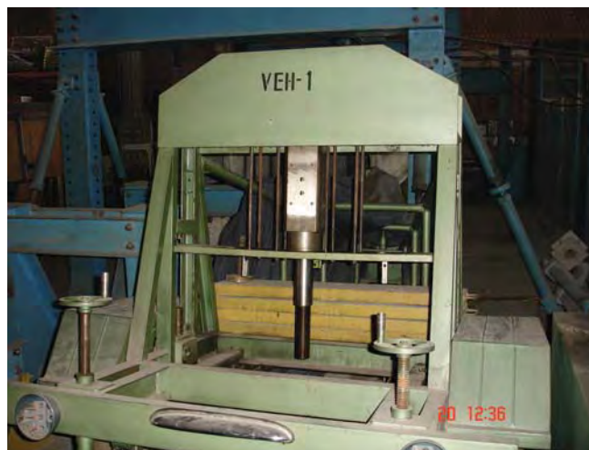
Figure 1. The electrodynamic vibrator built by professor Varlam from the Bridges Laboratory of the Faculty of Civil Engineering in Iasi.
